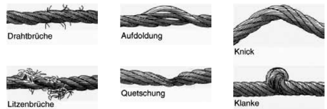
Fig. 37 Rope damage
